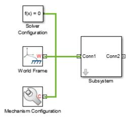
3 Right-click the Subsystem block, and select Mask > Create Mask. A mask editor opens up, enabling you to specify the numerical values of the MATLAB variables you entered in the Solid and Rigid Transform block dialog boxes.
