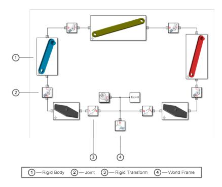
While important, rigid body subsystem and joint blocks are not sufficient to represent the four-bar linkage. Other blocks serve important purposes. These include World Frame, Rigid Transform, Mechanism Configuration, and Solver Configuration blocks. The table summarizes their functions in a multibody model.
