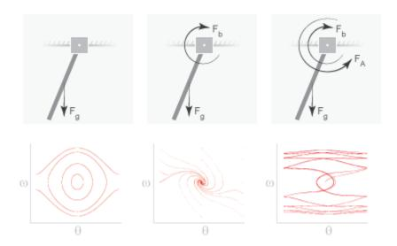
Your starting point is the simple pendulum model that you built in "Model Simple Pendulum" on page 1-19. By adding forces and torques to this model, you incrementally
