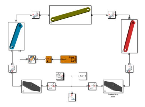
To specify the force or torque acting at a joint, SimMechanics provides a selection of actuation inputs directly in the joint blocks. Each joint primitive—the basic component of a joint block—provides a selection of actuation inputs specific to that primitive.
